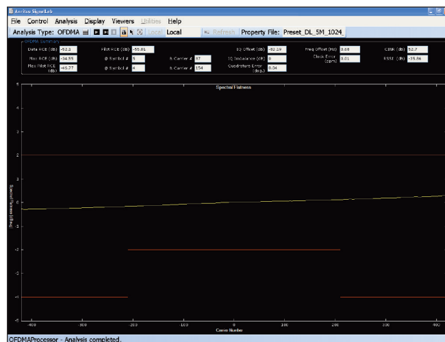
Figure 6. In a spectral flatness measurement, the power of the spectral lines is compared to a reference, such as the total transmitted power in a burst, to determine transmitter compliance to the WiMAX standard.
