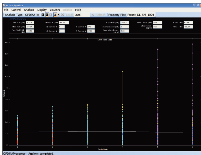
Figure 8. For evaluating trends in EVM performance, this plot of EVM as a function of time can help isolate events of interest.
